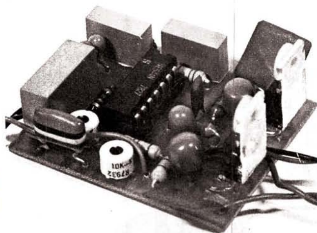
The component side of the finished p.c.b. without the heat sink. Compare this with the photographs of the prototype unit shown on the previous page
