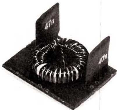
The radio frequency interference (r.f.i.) filter showing the bifilar wound toroidal inductors and the way in which the unit can be built on a small piece of Veroboard
